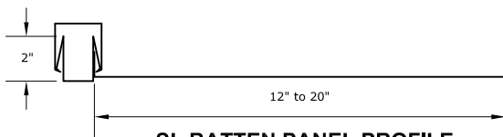
SL BATTEN PANEL PROFILE Standard Width(s)- 17"
